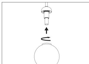
Carefully place the glass globe over the light bulb. Turn clockwise to attach the glass globe.
